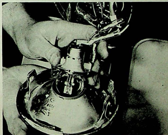
7.1b ... and unclip the bulbholder to replace the bulb
