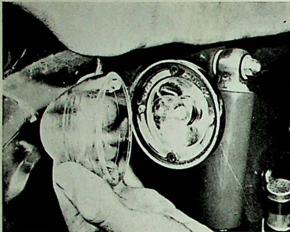
9.2 Remove two screws and plastic lens to replace bulb
