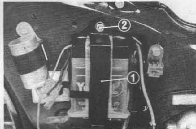
1. Battery band 2. 6 x 12 mm bolt
